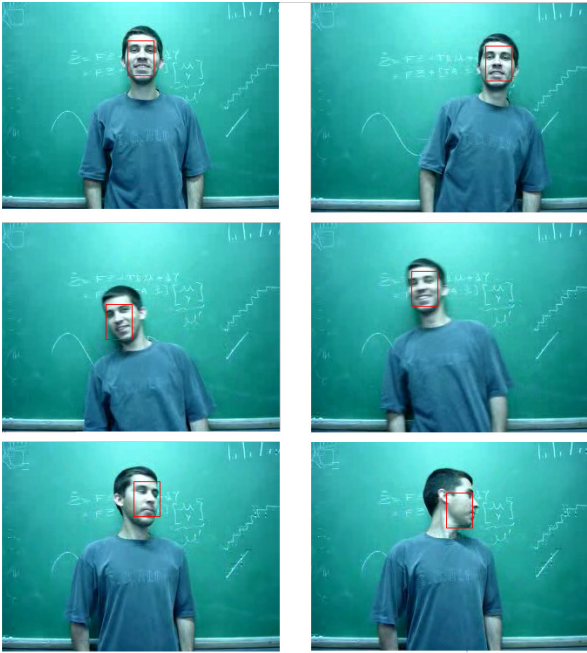
Figure 3. Six snapshots (frames 2, 60, 200, 300, 1000 and 1300, in a zig-zag sequence) of the face tracking in the video sequence 2, which shows face rotation and vertical displacement.
