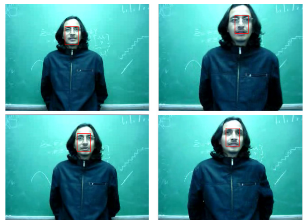
Figure 2. Four snapshots (frames 1, 220, 300 and 2000 in a zig-zag sequence) of the face tracking for the video sequence 1, showing the scale and light changes.
