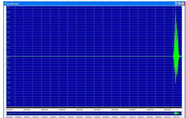
Figure 5. Output signal from the echo suppressor.
