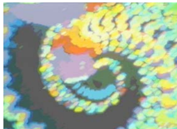
Fig. 8. Obtained result of image from Fig. 7 dilated by a 9x9 square structuring element through the developed hardware.
